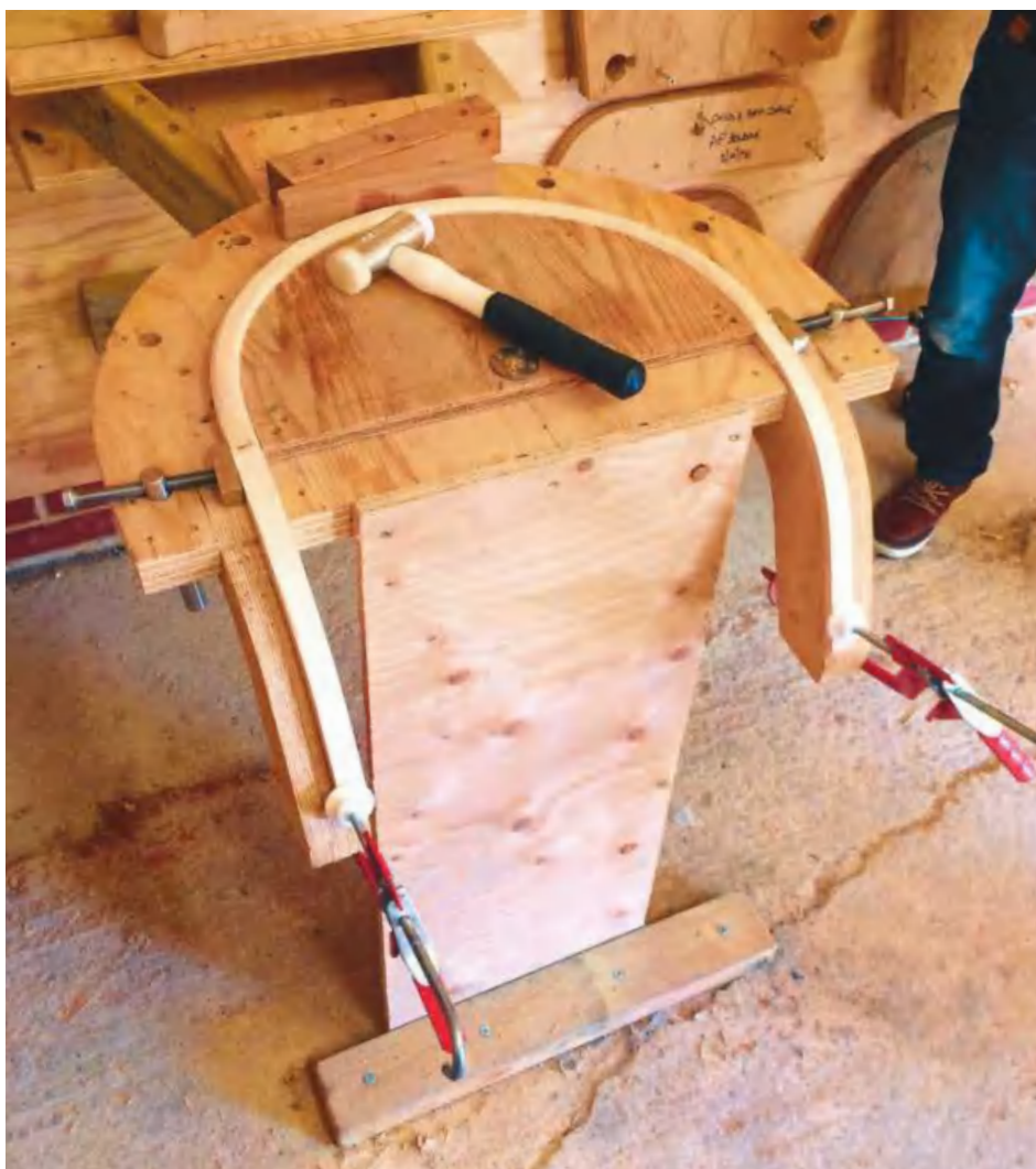
▲ Pic.7 ...the steam-bent hoop being allowed to set in the shaped former
